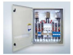
Series powerline protection is the best available protection for sensitive electronics such as rectifiers, switchmode power supplies, and other mission critical equipment. The Series Filter reduces the rate of rise of any transient overvoltage to acceptable levels, and also reduces the overall magnitude of the transient voltage the equipment receives.
